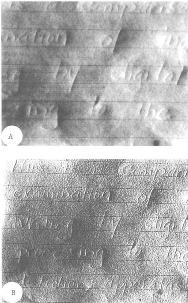
FIG. 4a—Photographs of ST 1 through ADIPS. (A) is ST 1 viewed through ADIPS camera with side lighting alone. (B) is enhanced image.
