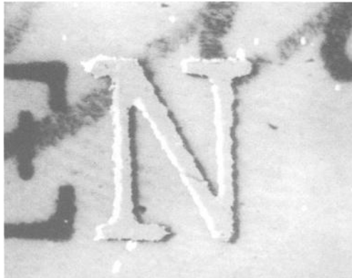
FIG. 8— Superimposition of film ribbon over typed letter, set off to the side.
